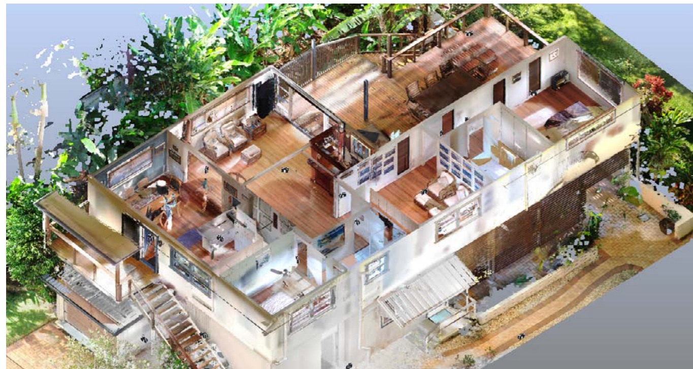
A 3D laser scan model of an older style beach house that has had numerous additions and modifications made over the years.
